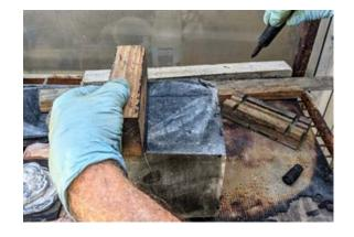
Cuts must be straight with subsequent cuts perpendicular to the first cut.
